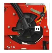
Each type of seed needs the appropriate seed disc (2, Fig. 3.8), since the seed's size, spacing between plants, etc, require specific discs with specific number of holes to control the distance between planted seeds. Besides, the holes need to be big enough to contain a single seed.
