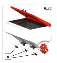
To **EMPTY** the fertilizer hoppers, open the caps placed on the hopper's lower part (A, Fig. 8.2).
